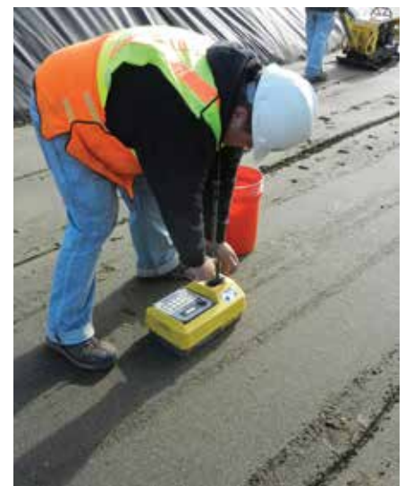
Testing material density.
