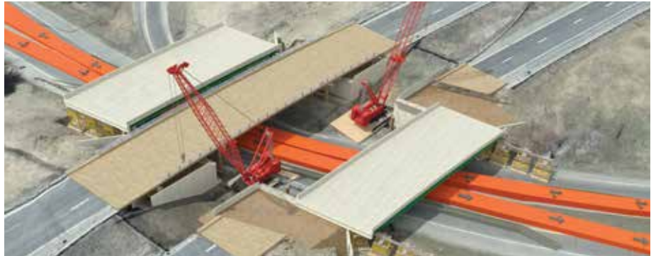
HARTFORD. Rendering of "Lateral Slide" bridge replacement project on I-91. Sliding in completed structure reduces duration of lane closures.
