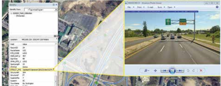
The Overhead Sign Structure Project uses Geospatial Information Systems to link data and imagery to more effectively catalogue overhead signs.
